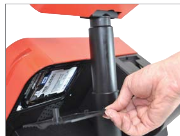
Easily Removable HDD (1 Screw)
