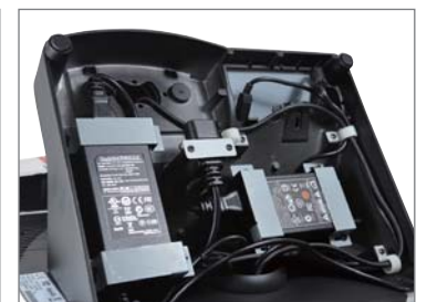
Separate Power Supplies for The Printer and The Terminal
